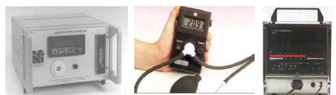
Fig. 8: Various types of residual oxygen measuring instruments (left: PBI-Dansensor – centre: Huntingdon Fusion – right: Orbimatic)
