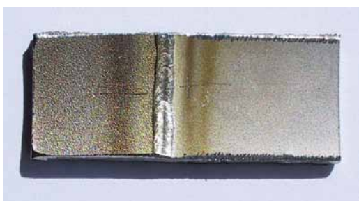
Fig. 9: Typical condensation film next to the weld, referred to as the 'manganese streak'
