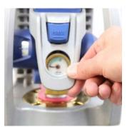
1. To shut off the valve slowly lower the actuator lever (E) to its closed position, ensuring it engages with the safety interlock mechanism (D).
