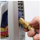
3. Disconnect the outlet hose connection (C) when the cylinder is empty or a different gas is required. The cylinder package is now safe to be stored or transported ahead of its next intended use.
