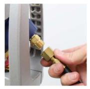
1. Remove light blue plastic cap from threaded valve Connection (B). Connect the relevant outlet hose connection (C). DO NOT OVER TIGHTEN.
