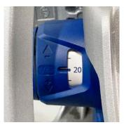
3. Slowly turn the flow control knob (F) in a clockwise direction to increase gas flow to the desired level (litres per minute) shown on indicator (G) at the notch. The EVOS VIPR is ready to deliver gas.
