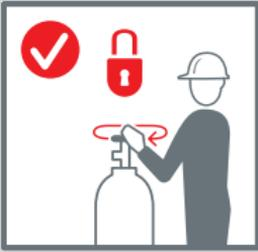
Close the cylinder shut-off valve.
