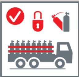
Ensure cylinders are fixed and secure before starting your journey, in an upright, vertical position and separated from the driver's compartment.
