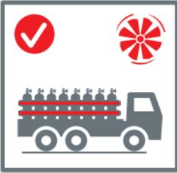
Use a well-ventilated vehicle, ideally an open or flatbed truck, or a vehicle with a purpose-built, sealed cabinet that is vented to the outside.
