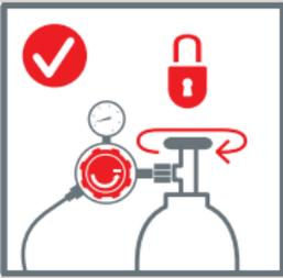
Don't rely on regulators or other gas equipment to shut off the gas. Remove regulators or other gas equipment from acetylene cylinders prior to transporting or storing cylinders.
